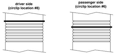
On Tundra Access Cab 4x4 V8 models, it is recommended that the driver side circlip is installed two positions higher than the passenger side circlip (Note: Do not use circlip locations #7 and #8 on Tundra Access Cab 4x4 V8). For example, to achieve the highest lift setting of 1" on a Tundra Access Cab 4x4 V8, the circlips should be installed as follows:
